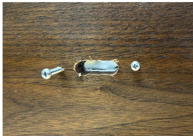
Markings left by spinning the screws into the holes.
