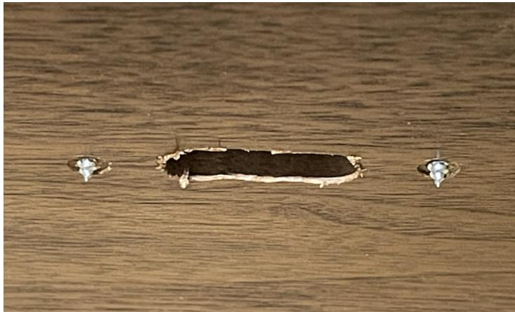
With a #1 hand philips screwdriver, use the screws to pre-tap the mounting holes in the bezel. Place a finger over the area directly in front of the screws path on the bezel front. When the screw bottoms out, it can usually be felt through the plastic. (Another mounting option is to drill completely through the bezel and use a nice-looking screw from the front. This is if you do happen to break through. Or call us for a replacement display.)
