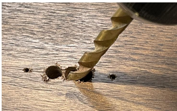
Example of finished drilling to provide an opening for the display to pass through and the mounting screws to protrude through.
